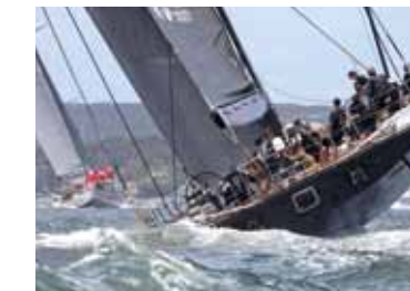
WITH COMANCHE Given that Wild Oats XI 's stern can fit twice into Comanche 's it's hard to believe that the two boats were so evenly matched. But when Comanche heels at 25° she has the same wetted surface as Wild Oats . The latter's narrower cross section allows her to gain mileage from VMG running
