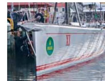
BOW The refairing of the bow section, remodelling of the bowsprit and lifting of the bobstay attachment to the stem have streamlined the forward end of the boat and made it drier for the bow team. Photographers are the only losers
